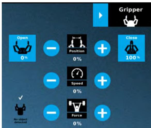
Fig. 7: GUI of the Robotiq gripper
