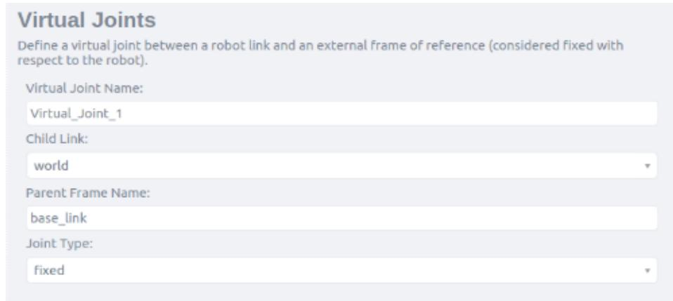
**IMPORTANT:** Make sure that the options are exactly as specified. Then click the Save button, now the robot should spawn, and you should see this window:
