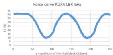
Fig. 16. Force curve of the KUKA LBR iiwa with bad parameterization of the impedance controller.
