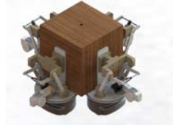
(b) CAD view of four m-bots transporting a cubic payload on their top [17].
