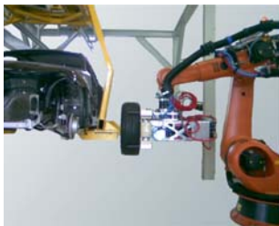
Fig. 5. Example of a force-controlled assembly process [21].
