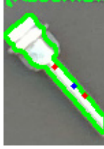
Fig. 11: Calculated gripping point (blue) for the assembled object. Upper left [red] is contour center and also one of the reference point and down right [red] point is another reference point which is adopted the highest distanced points from the contour center point.
