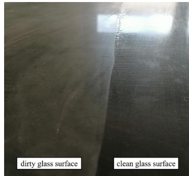
Fig. 4: dirty vs. cleaned glass surface
