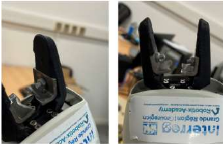
Fig. 4 Proposed clamp mounted on the robot
